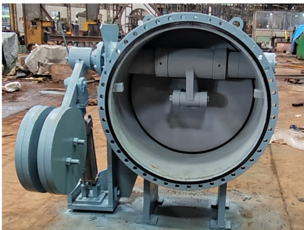
DN 1000 MM Jansen Type Dashpot Check Valve supplied to a Large Fertilizer Plant
