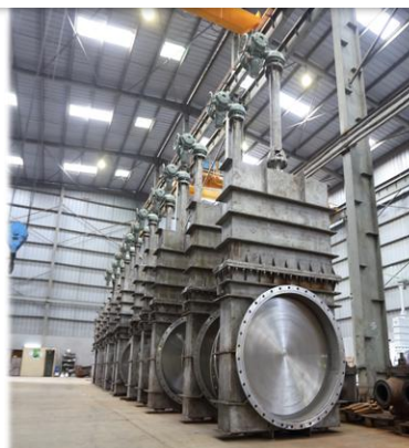
34 Nos of DN 1400 MM Double Disc Gate Valves supplied to SAIL BSL for Ammonia Sulphate Plant
