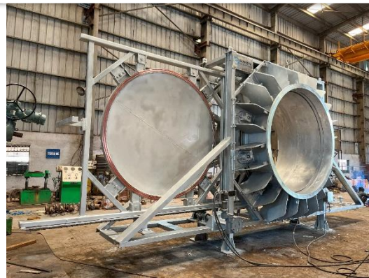
DN 2800 MM Fabricated Butterfly Valve manufactured & supplied to JSW Steel Ltd, Dolvi, for Blast Furnace Application
