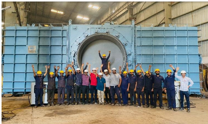
3 Nos of Double Disc Gate Valves sized DN 2500 supplied to JSW Steel for EMD Project
